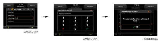
· The logged faults of the MCU, engine ECM or AAVM (option) can be deleted by this menu.
