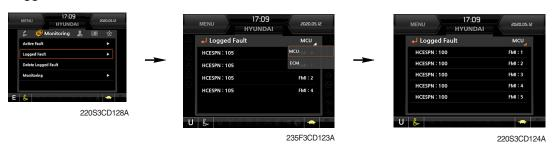
· The logged faults of the MCU, engine ECM or AAVM (option) can be checked by this menu.
