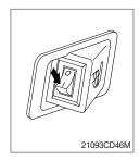
(1) This switch is used to heat the seat.
