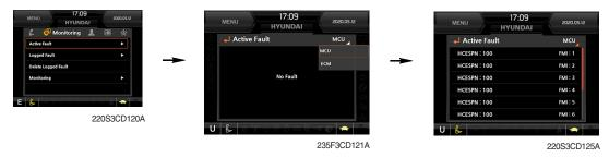
· The active faults of the MCU, engine ECM or AAVM (option) can be checked by this menu.
